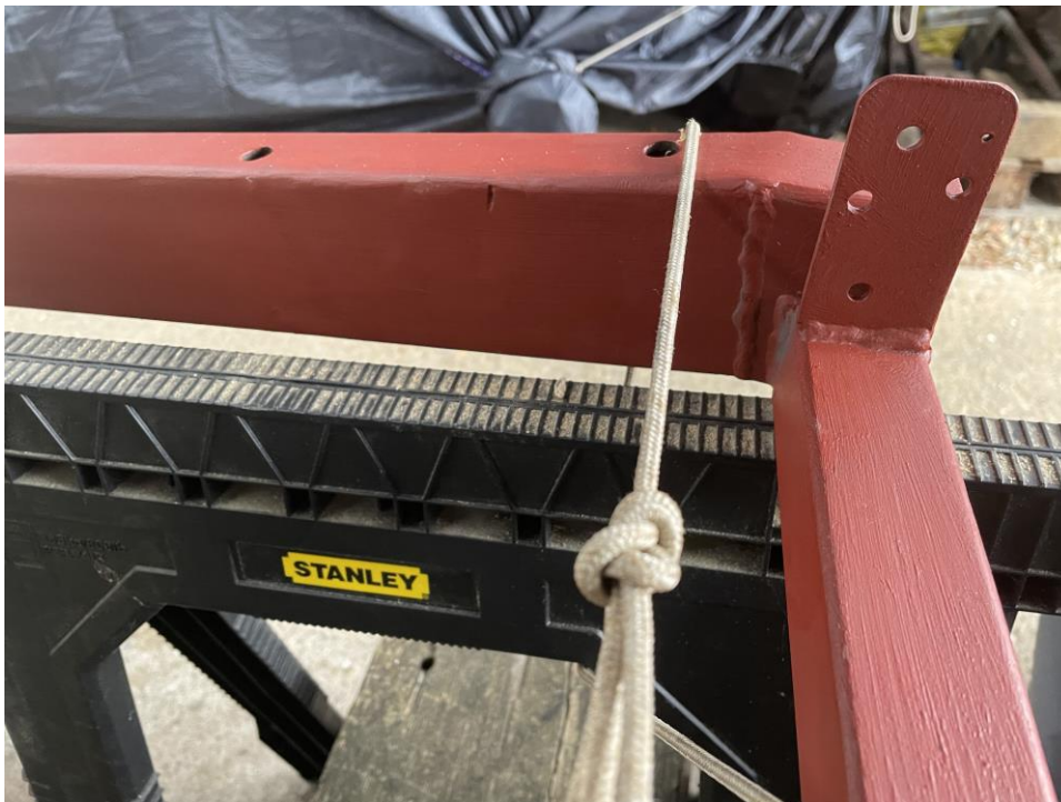
Chassis sans left hand front engine mounting bracket.
