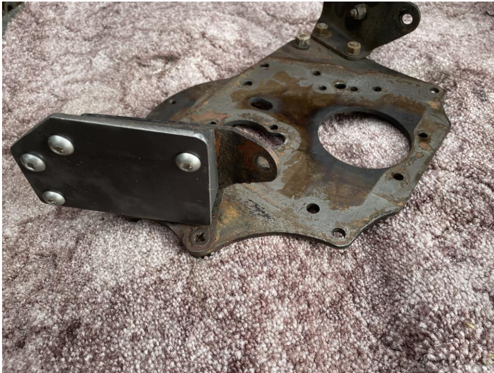
The new flat plate is fitted to the rubber mounting.
